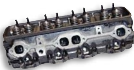
FAP1600E91 NEW 5.7L Cylinder Head - GM, V-8 Chevy Pre-Vortec 1987-95 cylinder head, accepts 12-bolt intake manifold (4 inside intake manifold bolts @ 23 degrees), center-bolt valve covers. Valves & springs included.
