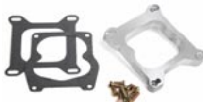
717-6 Cast aluminum adapter that will allow any 4150 or 4160 carburetor to be mounted on manifolds designed originally for Rochester Quadrajet or Carter Thermo Quad carburetors. This adapter can also be used in reverse
